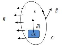
The magnetic flux through a small area "dS" will be  $\overline{B}$ . Now the flux through the entire circuit is
