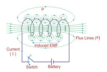
Consider a coil connected to a battery through key (k). When the key is closed, due to increasing current in the coil, the magnetic field and hence flux linkage with the coil also increases. As a result of this, induced emf is set up in the coil. According to Lenz's law, the direction of induced emf is such that it opposes the growth of current in the coil. This delays the current to acquire the maximum value.
